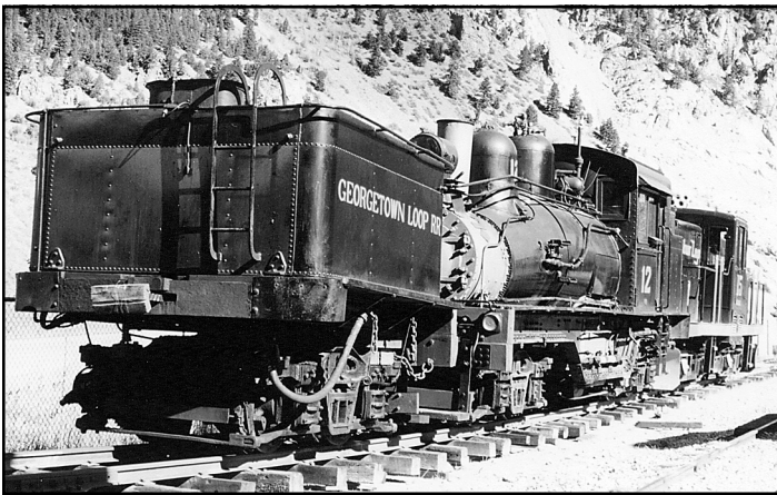
GLRR Shay #12 is on the loading ramp track at Silver Plume. The tender has been swapped to the front to be put on a trailer first. General Electric built diesel #15 pushes them, and will be the last loco to leave. – October 28, 2004, photo © Dave Schaaf.
